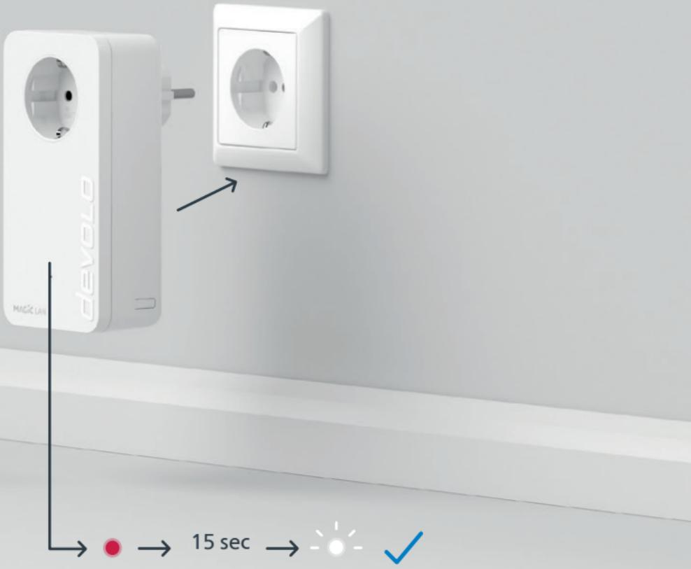
**| EN |** Connect the devolo Magic LAN adapter to a free wall socket and wait until the LED quickly flashes white (approx. 15 sec).
